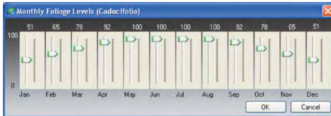
Figure 13. It shows the position of the sliders for a tree species that begins the year with 51% of its foliage, reaches its maximum foliage (100%) between May and August and then gradually experiences a decrease in foliage until it again reaches 51% at the end of the year.
